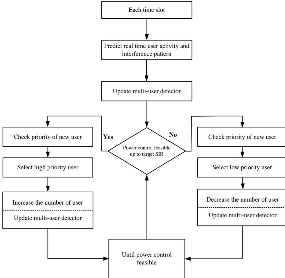
**Fig. 6.** Block diagram of prioritized resource allocation based power control method.
