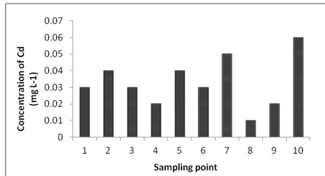
**Fig. 8.** Cd concentration at different sampling points.
